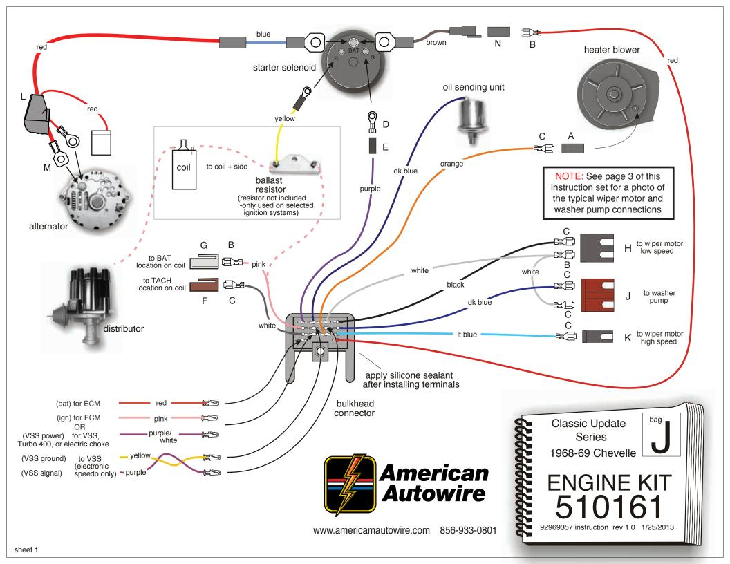
TEMPORARILY, PLUG THE MAIN BULKHEAD CONNECTOR ON THIS HARNESS INTO THE MATING DASH BULKHEAD PLUG AT THE FIREWALL (LOCATED UNDER THE MASTER CYLINDER) AND TIGHTEN THE BOLT TO SEAT THE CONNECTOR. (Note: This will be unbolted and removed to install the front lamp portion of the harness at a later time. Once you have completed your installation, we recommend sealing all outside cavities with black RTV silicone sealant and coating the inside of the connector cavaties with die-electric grease.)
