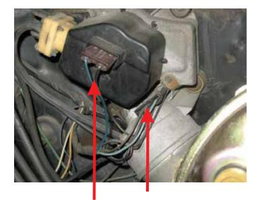
The photo above depicts the typical stock 1968-1969 Chevelle or El Camino wiper motor and washer pump connections with a "depressed park" motor (hidden wipers). Where you see a black wire with a yellow stripe in the photo (red arrows), that would be equivalent to the AAW white "wiper feed" power wire.
